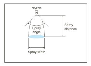
The spray angle is measured at the top of the spray made by straight lines extending along the outer edges of the spray.
