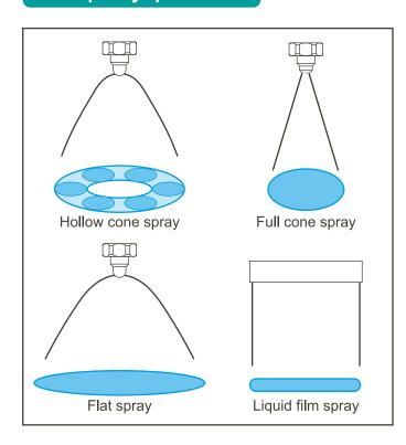
Spray pattern means the cross sectional shape of spray.
