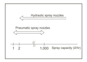
The spray capacity is the water volume flow rate sprayed from the nozzle. One of the features of pneumatic spray nozzle is to spray at extremely small capacity such as 1.7 cc/min. or 0.1  $\ell$ /hr.
