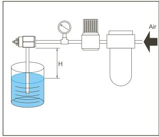
Spray capacity differs depending on liquid siphon height (H).
